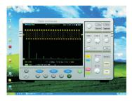
The functions of Micsig's ScopeSuite software include upgrading, real time control, measurement, storage, dynamic display, record, and data analysis.
