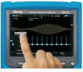
Three operation modes for moving waveform, zooming in and out, and using menu by touch, button and scroll wheel.
